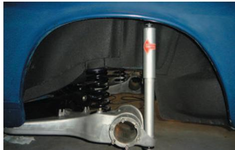
Next up, we should have the diff installed as well as our newly conditioned rear axles. We will also rebuild the power steering rack and run the new brake lines. This all looks so cool, that it seems almost a shame to put the wheels on.
